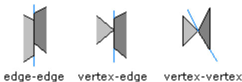
Figure 2. Edge-edge contact (left), vertex-edge contact (middle), and vertex-vertex contact.
